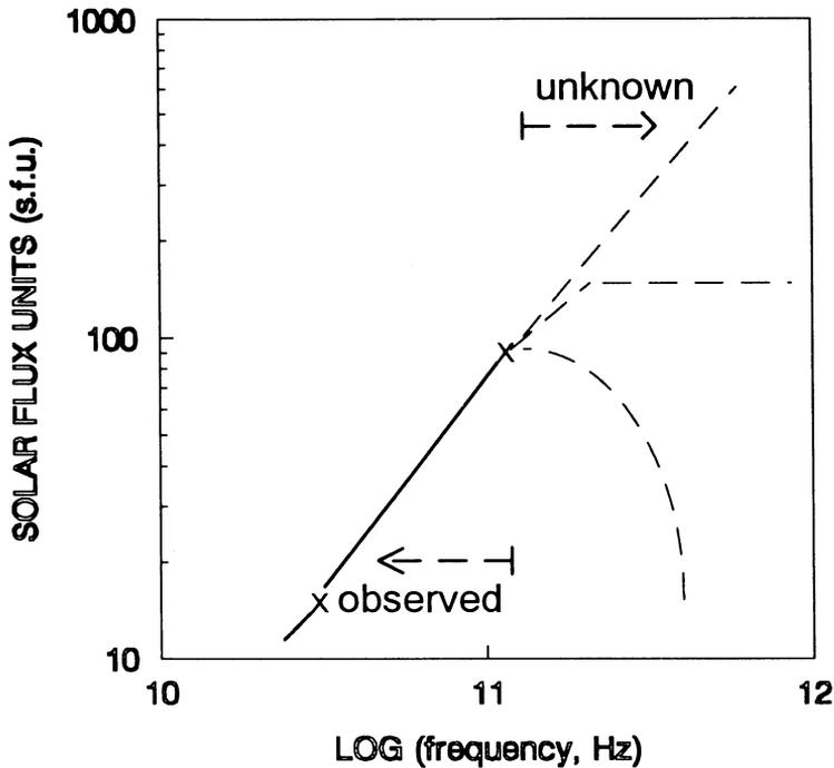
Fig. 3. Possible spectral behavior at frequencies above 100 GHz.
