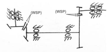
Figure 3. Principle sketch of a two-stage gearbox (WSP)
