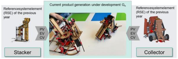
Figure 4. The system in MSuP consists of two subsystems: a moving system, which collects cubes on a board (collector), and a standing system, which stacks the cubes into towers (stacker).
