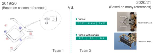
Figure 1. Solution concepts of the teams of the two cohorts for the first milestone of the Live-Lab MSuP. E: Effort, R: Risk, B: Benefit WS: Winter semester MS: Milestone. The purpose of the shown systems is to collect cubes autonomously driving on a playing field in order to pass them later to a second subsystem.
