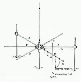
Fig. 6. The star ablatometer.
