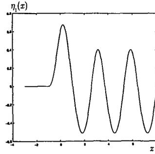
Figure 8: Hydraulic fall solution,  $\eta_1=0$  for  $x \leq -1$ ,  $\lambda = -0.79169267$ .
