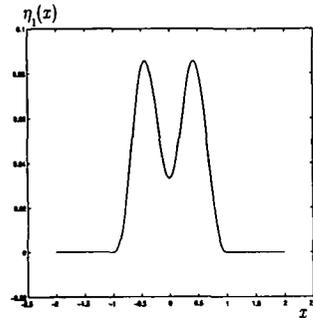
Figure 11: Symmetric wave solution with one humps,  $\eta_1(-1)=0$  for  $x \leq -1$ ,  $\lambda = -6.1258501$ .
