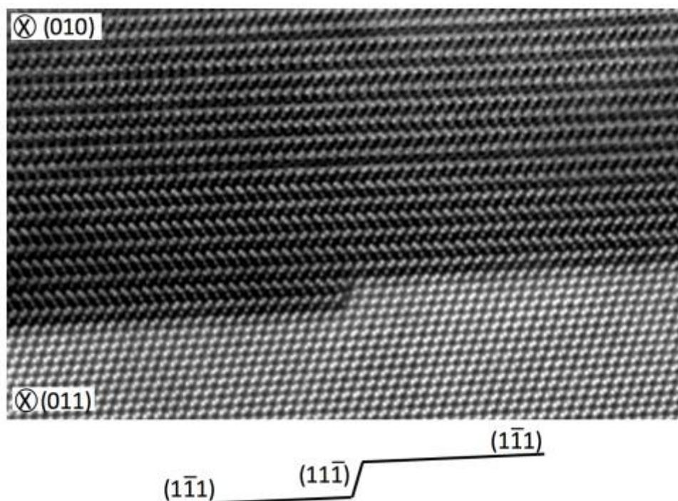
**Figure 1:** Probe corrected HR-STEM image, corrected for non-linear scan distortion. The bottom of the image is the MBE grown Ge layer, with the CaGe<sub>2</sub>
