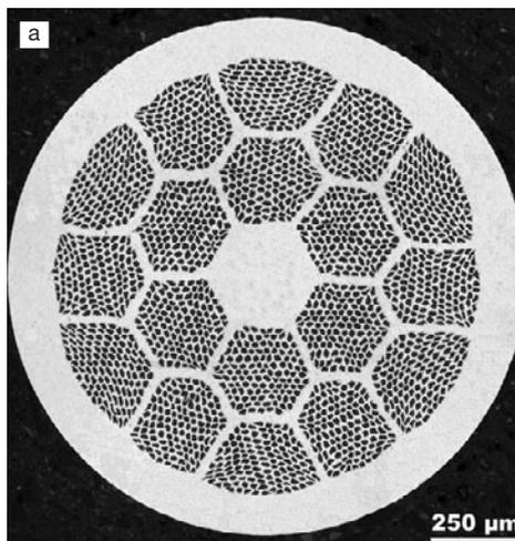
(a) Cross sections of the round wire Bi-2212 multifilament conductor before reaction, and (b) electron backscatter diffraction images of the grain structure after reaction at a high current density state. Major misalignments shown by the red-colored grains exist without preventing high filament current densities. Credit: Jianyi Jiang and Fumitake Kametani.
