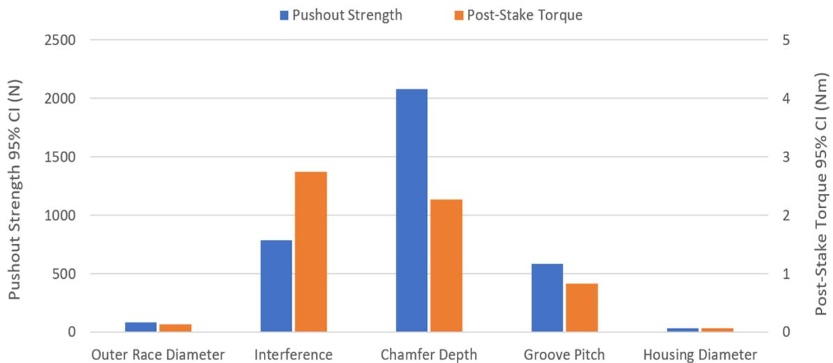
Figure 6. Impact of manufacturing tolerances
