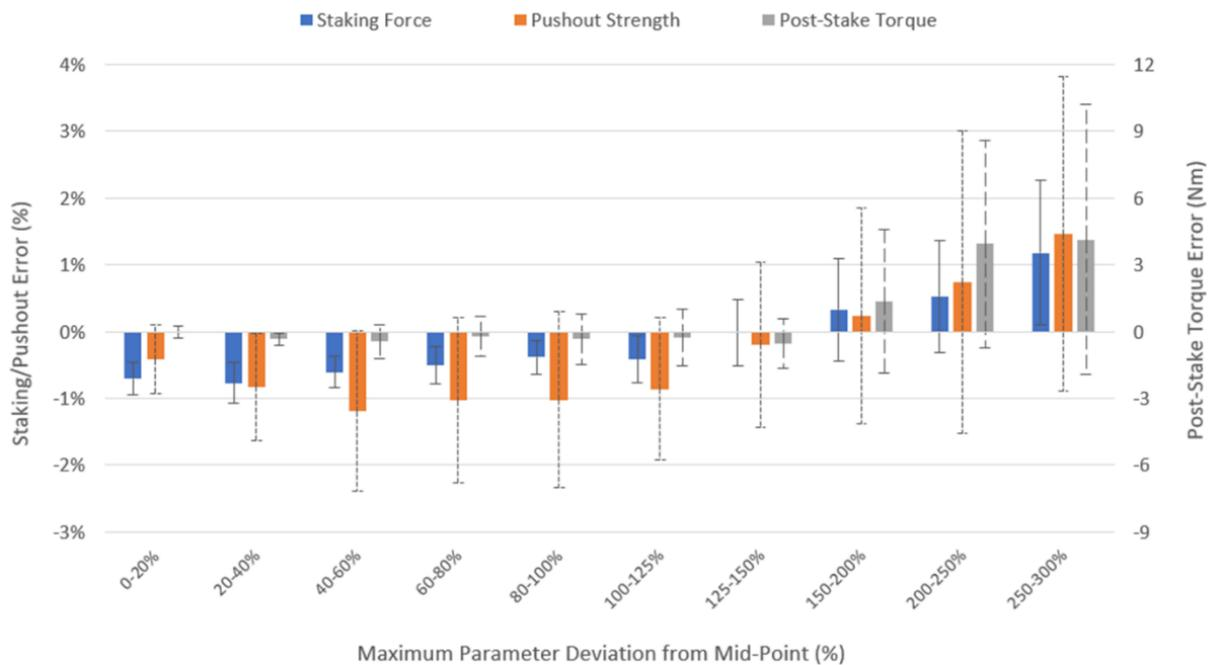
Figure 4. DOE model error with 95% confidence intervals.
