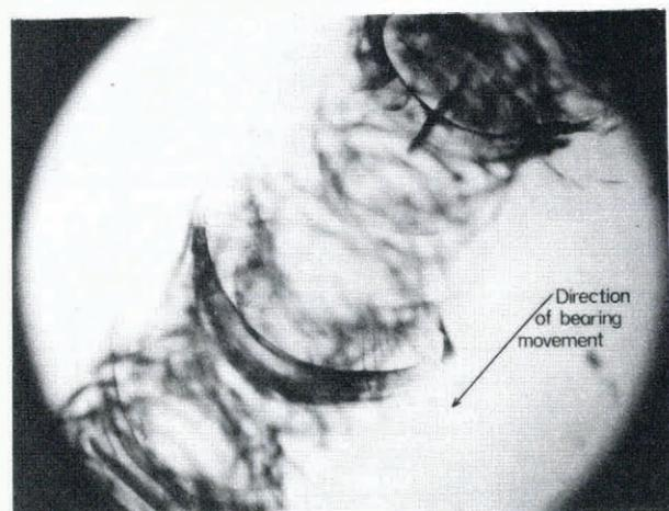
Fig.4. As Figure 3 but with focus altered to show convex-forward cracks more clearly.
