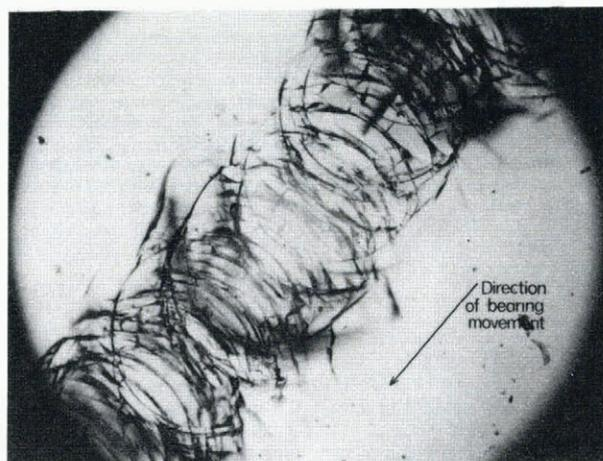
Fig.3. Trace made by non-rolling bearing under relatively high pressure (x25 magnification).
