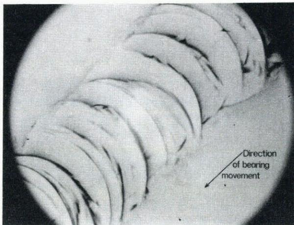
Fig.2. Trace made by non-rolling bearing under relatively low pressure showing concave-forward cracks (x 50 magnification).
