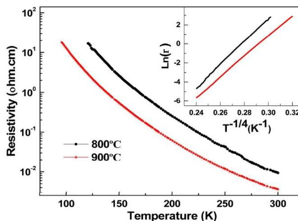
**Figure 2.** Temperature dependence of the electrical resistivity of the films grown at 800 °C and 900 °C. The inset displays a plot of  $\ln(\rho)$  versus  $T^{-1/4}$ .
