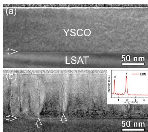
**Figure 1.** Low-magnification bright-field TEM images of the YSCO films grown at 800 °C (a) and 900 °C (b). The EDS spectrum of the second-phase particles is inserted in (b).
