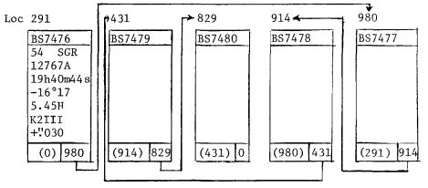
Figure 3. A list structure arrangement of the records in Figure 2. 0 indicates the end of the list. If the 0 were replaced by 291, this would be a ring structure. Backwards pointers are shown in parentheses.
