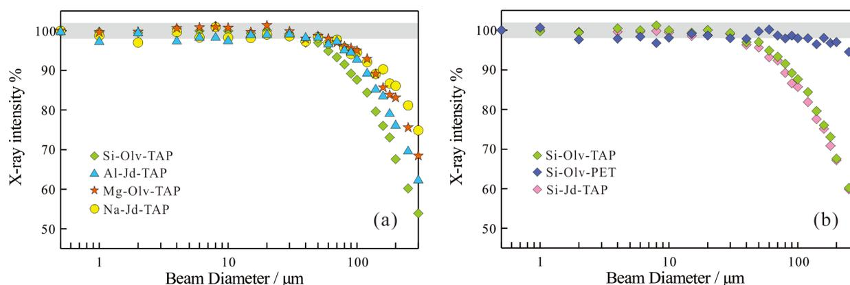
**Figure 1.** Graph showing with the increasing beam diameter, the detected characteristic X-ray intensity changes of (a) Na, Mg, Al and Si with a TAP crystal and (b) Si in olivine and jadeite with a TAP and a PET crystal. The gray area in the graph ranges from 98% to 102% on the vertical axis.
