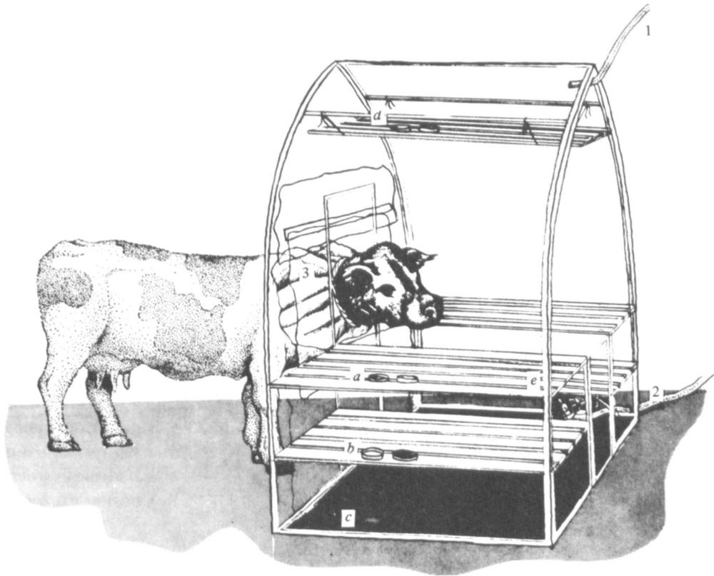
Fig. 1. Aerosol chamber in place for exposure of an adult bovine. 1 = exhaust hose, 2 = air pressure supply hose, 3 = neck sleeve of plastic sheeting, *a, b, c, d* = open Petri dish air samplers, *e* = location of May air sampler if used.
