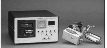
The Evactron <sup>®</sup> De-Contaminator with Oxygen Radical Source (ORS) mounts on your SEM or FIB.
