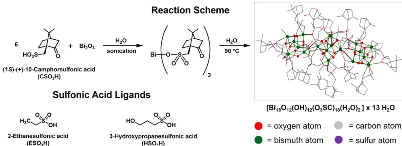
**Scheme 1:** Reaction scheme of the bismuth-oxo-cluster synthesis with (1S)-(+)-10-Camphorsulfonic acid (CSO<sub>3</sub>H) [6]. Two further sulfonic acid ligands are shown, which were used for synthesis. On the right the single X-ray crystal structure of the bismuth-oxo-cluster derived from CSO<sub>3</sub>H is displayed [6].
