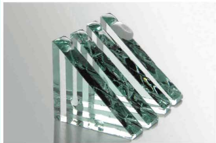
Fig. 1: Qwick glass knives having virtual water troughs are prepared by application of various hydrophobic substances including (left to right) pap pen, finger nail polish, histologic mounting medium, and paraffin. A water droplet added between the hydrophobic substance and the cutting edge of the knife provides a suitable water surface for the collection of sections cut from an epoxy-embedded tissue block.
