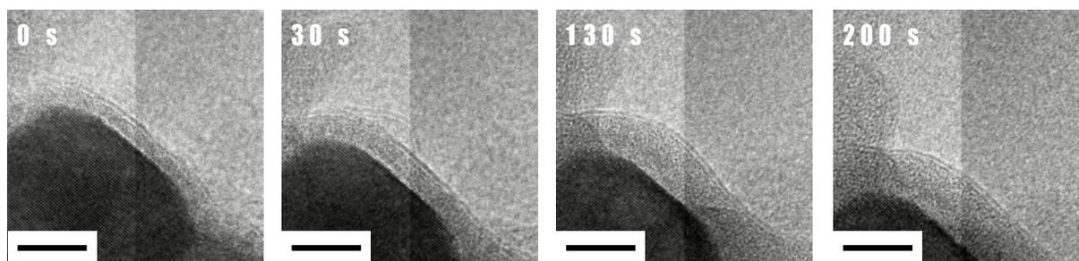
**Figure 2.** Time-series TEM snapshots of movie showing the formation of uniform amorphous layer on SnO<sub>2</sub> nanotube. (Scale bar = 10 nm)
