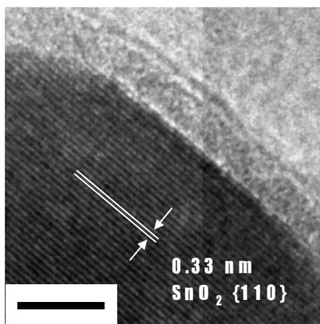
**Figure 1.** HRTEM image showing (110) plane of SnO<sub>2</sub> nanotube. (Scale bar = 5 nm)
