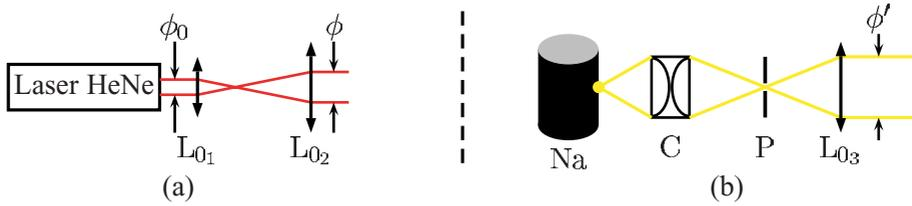
**Figure 2.** Sources used. (a): the afocal system formed by  $L_{01}$  (+5 mm) and  $L_{02}$  (+100 mm) lenses allows to enlarge the quasi-cylindrical beam emitted by the HeNe Laser. (b): the condenser C concentrates the beams coming from the Na Spectral Lamp on a pinhole P ( $\varnothing = 57 \mu\text{m}$ ) placed at the first focus of the lens  $L_{03}$ .
