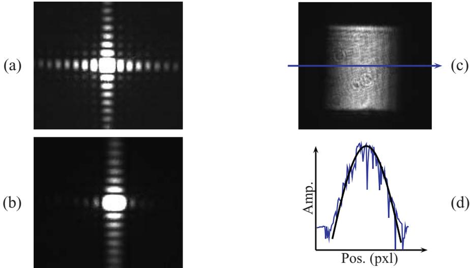
**Figure 3.** Example of results obtained with the Laser Source. (a): Non-apodized PSF obtained in the plane  $P_1$ . (b): Apodized PSF obtained in the plane  $P_2$ . (c)&(d) give respectively the distribution of intensity in the pupil plane  $P_3$  and its cut parallel to the direction of apodization.
