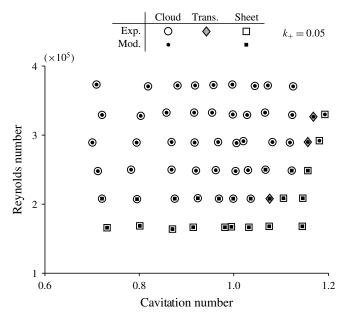
FIGURE 8. Stability map for sheet and cloud cavitation for  $k_+ = 0.05$ . The map shows operation points where sheet (squares) and cloud cavitation (circles) occur. Operation points marked with diamonds could not be categorised. The larger symbols mark the experimental data, the smaller symbols are the results of the physical model (experimental data by Pelz *et al.* 2014).
