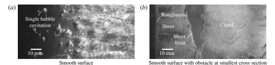
FIGURE 3. Single bubble cavitation (a) and transient cloud cavitation (b) in convergent–divergent nozzle from top view perspective. The flow is from left to right. The image shows a section of the divergent part of the nozzle. The surface bounded obstacle ( $\hat{k} = 1$  mm) is positioned 5 mm to the right of the left edge of picture (b). The cavitation number is  $\sigma = 0.228$  and the Reynolds number is  $Re = 4.2 \times 10^6$ .
