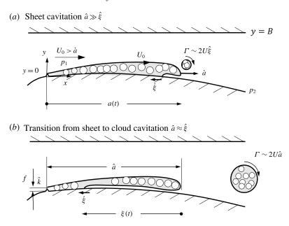
FIGURE 1. Sketch of sheet (a) and cloud cavitation (b).
