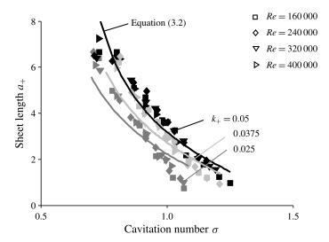
FIGURE 4. Sheet cavity length  $a_+$  plotted against cavitation number for four Reynolds numbers and three obstacle heights (experimental data by Pelz *et al.* 2014). The solid lines are calculated with (3.2) using the approach  $(fR_0/U_0)^2 = 0.97 k_+^{0.3}$ .
