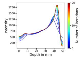
**Figure 4.** The iteration steps of the reconstruction algorithm shown as the laterally integrated 3D reconstruction signal plotted over the penetration depth for the 70 MeV Bragg peak (BP) reconstruction.
