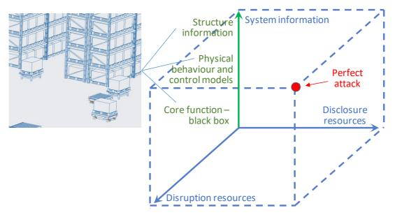
Figure 4. Three-dimensional model of an attack - the attack space
