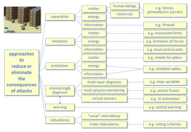
Figure 5. Approaches to reduce or eliminate the consequences of attacks
