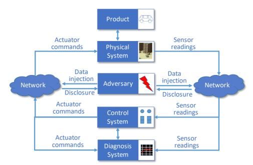
Figure 2. System model of an external attack to an automated system
