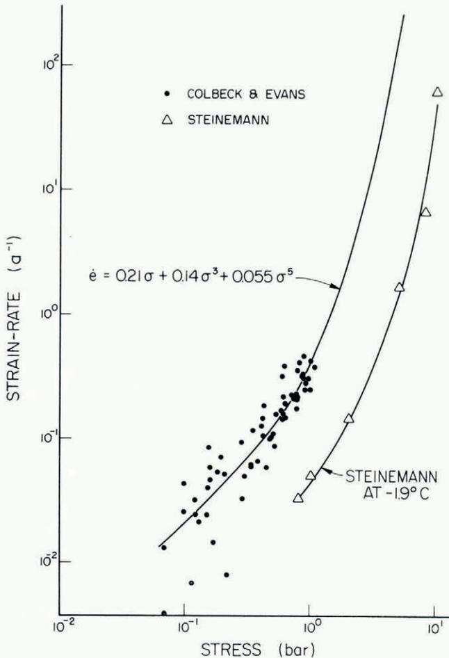
Fig. 7. Equation (6) and Steinemann's results.
