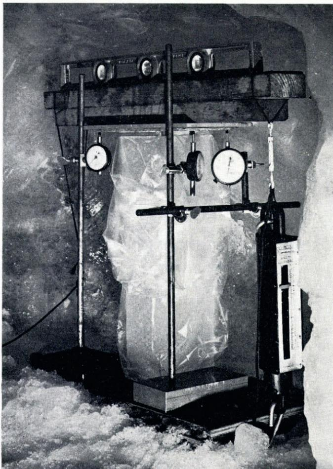
*Fig. 2. Compression test apparatus (photograph by E. R. LaChapelle).*
