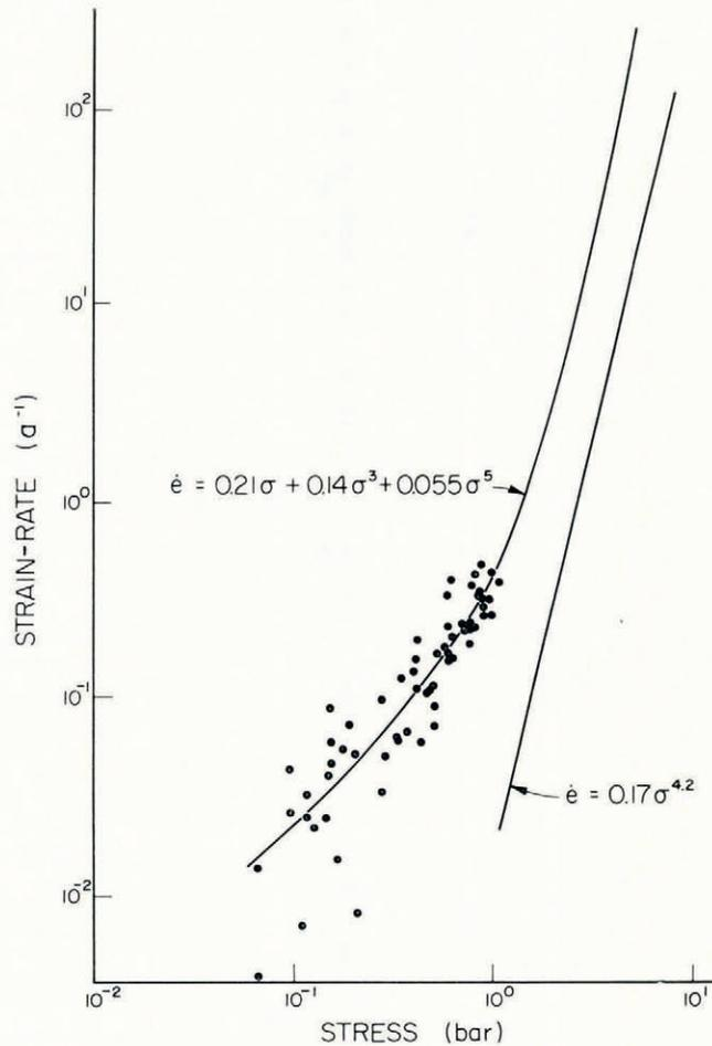
Fig. 6. Equation (6) and Glen's quasi-viscous flow law.
