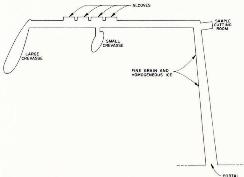
Fig. 1. Plan view of the ice tunnel. Scale 1 : 300.
