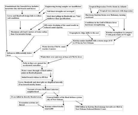
Figure I. A causal theory for the failure of the 17th Street canal levee in New Orleans during Hurricane Katrina. Sources: American Society of Civil Engineers Hurricane Katrina External Review Panel 2007; Bea 2008; Rogers et al. 2008; Boyd 2012.
