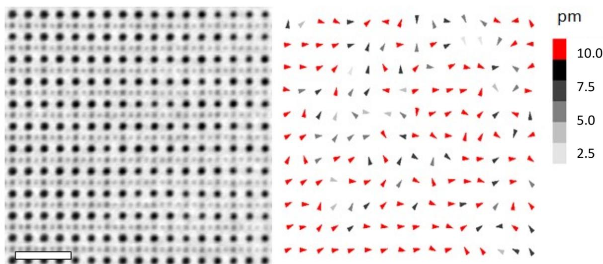
**Figure 1.** Experimental ABF-STEM image in [011] zone axis acquired at RT (left) and O vs Ti displacements in  $\text{Ba}_{0.6}\text{Sr}_{0.4}\text{TiO}_3$  sample (right). Scale bar is 1nm. Average absolute value of displacements was  $13.4 \pm 7.4$  nm.
