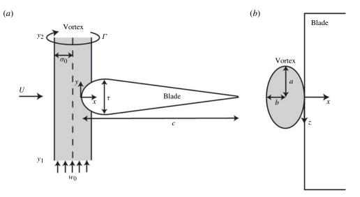
FIGURE 1. Schematic diagram showing the parameters used to describe the vortex cutting problem and the control volume (shaded) used in the scaling analysis, from both (a) the side view and (b) the top view.
