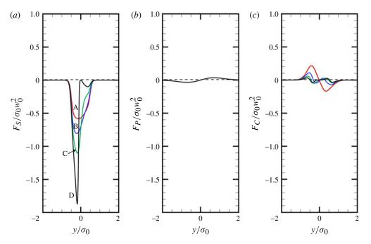
FIGURE 3. Plots showing variation along the vortex core of (a) the shear force  $F_S$ , (b) the pressure gradient force  $F_P$  and (c) the vortex circulation gradient force  $F_C$ , per unit mass, at times  $w_0 t/\sigma_0 = 0$  (dashed), 1 (A, red), 2 (B, blue), 3 (C, green) and 4 (D, black), for the same case as shown in figure 2. The pressure gradient force does not change in time.
