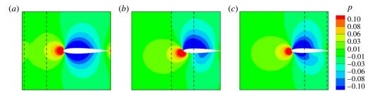
FIGURE 11. Time series of pressure contours in the x-y plane for Case 5 at (a) t = 1.8, (b) 4.2 and (c) 6.6. Edges of the vortex core are indicated with dashed lines.
