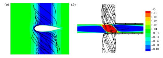
FIGURE 9. Contour plots from Case 13 of  $\omega_y$  (*a*) in the *x*-*y* plane and (*b*) on the blade surface projected onto the *y*-*z* plane, viewed from a perspective looking in the *x*-coordinate direction, at t = 6. Vortex lines in both the vortex core and blade boundary layer are plotted in black.
