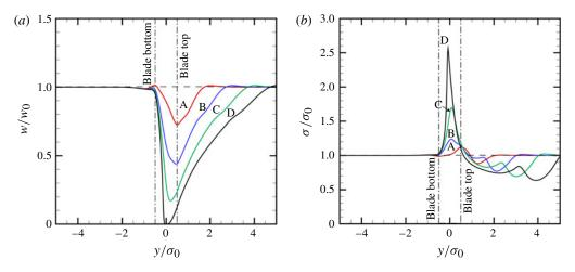
FIGURE 2. Computational results for (a) vortex axial velocity and (b) effective core radius from the plug-flow model for a case with dimensionless parameter values I = 1, A = 2, T = 1 and  $Re_A = 500$ . The plots are drawn for times  $w_0 t/\sigma_0 = 0$  (dashed), 1 (A, red), 2 (B, blue), 3 (C, green) and 4 (D, black), where the last time coincides with the vortex cutting time.
