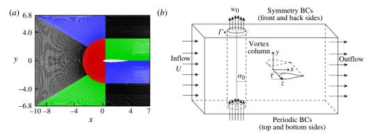
FIGURE 5. (a) Cross-sectional view of the computational grid in the plane z = 0 and (b) schematic diagram showing boundary conditions, as used for the full Navier–Stokes simulations. The inlet and outlet planes are at x = -10 and x = 7, respectively, and the blade span length is equal to 10.
