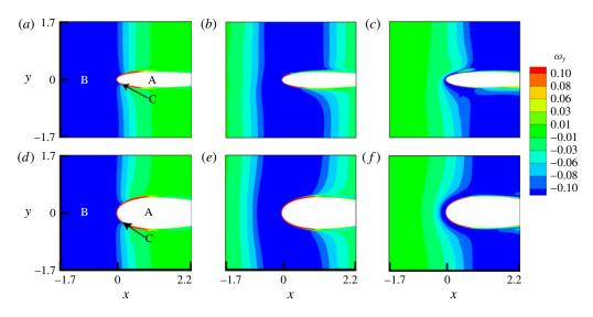
FIGURE 8. Contours of the vorticity component  $\omega_y$  in a plane z = 0 along blade leading edge for cases with thickness parameter values T = 0.48 (Case 5, a-c) and T = 1.05 (Case 13, d-f) at times (a,d) t = 3.6, (b,e) 4.8 and (c,f) 6. The blade cross-section is labelled as A, vortex core as B and blade boundary layer as C.
