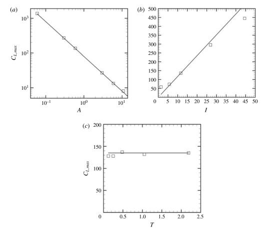
FIGURE 14. Variation of the maximum value of the lift coefficient with (a) axial flow parameter (I = 11.6, T = 0.48), (b) impact parameter (A = 0.6, T = 0.48) and (c) thickness parameter (A = 0.6, I = 11.6). Symbols are results of full Navier–Stokes computations and lines coincide with the prediction of the scaling result (5.4).
