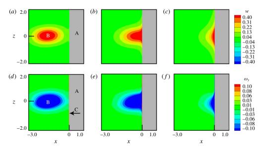
FIGURE 7. Time series from Case 5 showing contours of axial velocity (a-c) and axial vorticity (d-f) in the blade symmetry plane (y=0) at times (a,d) t=2.88, (b,e) 4.08, and (c,f) 5.28. The blade surface is labelled as A, vortex core as B and blade boundary layer as C.
