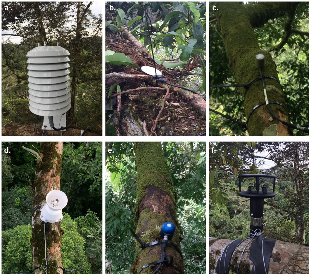
Figure 3. Set of sensors used to monitor climate with a 10-min temporal resolution in the tropical rainforest canopy of Yasuni National Park, Ecuador. In each station, a radiation shield (a) protected the sensor for temperature and relative humidity from direct sunshine and rain. The leaf wetness sensor (b) and the sensor for photosynthetic active radiation (c) were placed on the upper side of the medium section of a crown branch. Selected canopy climate stations were instrumented with a generic rain gauge (d), a sensor for global radiation (e), or a digital anemometer (f), as indicated in Table 1 . Instrument details are provided in Table 3 .
