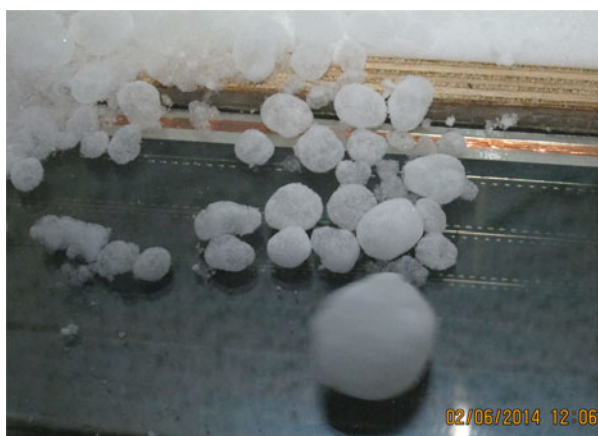
Fig. 5. Slightly melted yukimarimo accumulated inside the enclosure of the lidar heated glass window (height, 6 m).
