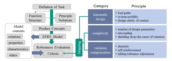
Figure 2. Robustness evaluation of product concepts utilizing the EFRT-model and criteria based on RD principles adapted from Goetz et al. (2019)
