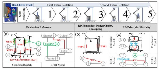
Figure 4. Application of mapping between robustness principles and information in EFRTmodel using the example of a coining machine.
