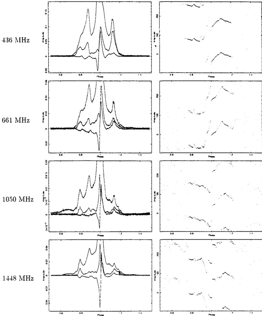
Figure 1. Polarimetric observations of PSR J0437–4715 at four different radio frequencies. The plots on the left show the profiles in Stokes I, L and V with arbitrary absolute scales. Stokes I is the upper curve in each plot and is clipped to show the low level emission. In all cases Stokes V is the lowest curve of the three. The plots on the right show the position angle of the linear polarization. The position angle is shown twice in the range  $(-90, 270)$  deg to assist the eye.
