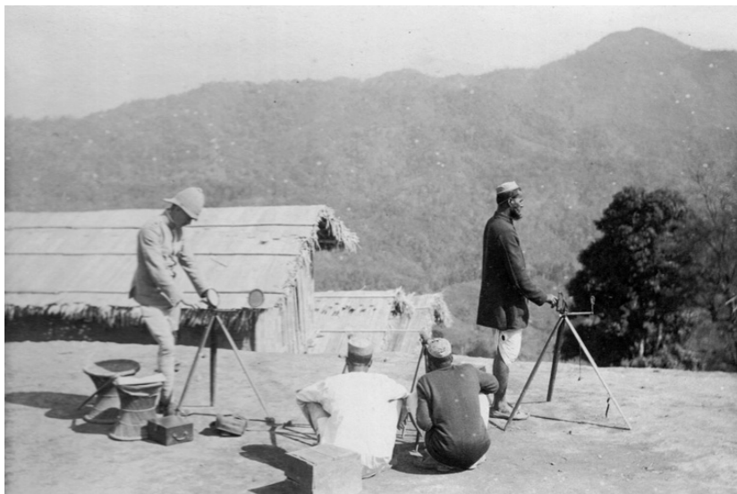
Figure 1.6 Signalling by heliograph towards an outpost at Lalbura's defeated village, c. 1892. Kwantlen Polytechnic University Special Collections (hereafter KPUSC), G 155 A1 P46 1893.
