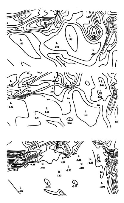
Figure 2: (top) density, (middle) temperature, (bottom) vorticity, at t = 2.5 for a flow with an initial Mach number of 2, and  $r_m = 1.7$ .
