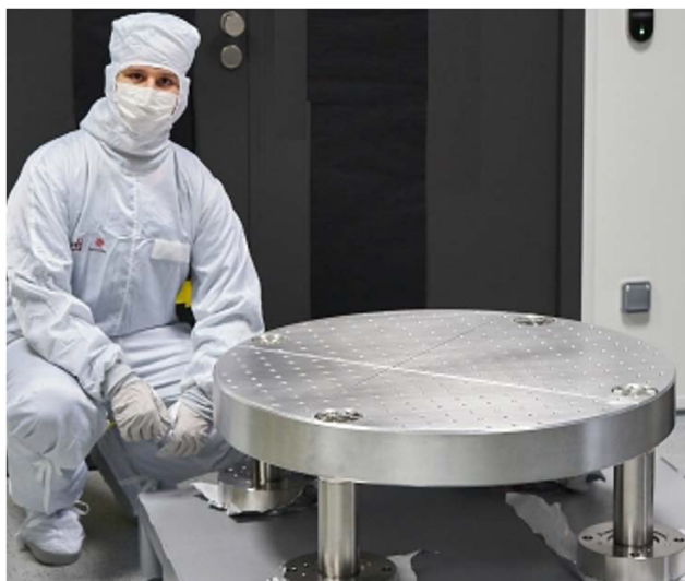
Figure 9. Photo of the 100 mm thick aluminium breadboard with its four monolithic stainless-steel legs.
