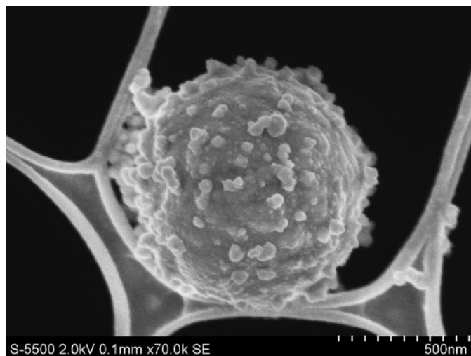
Figure 2: Secondary electron image of a typical GSR particle showing associated smaller particles.
