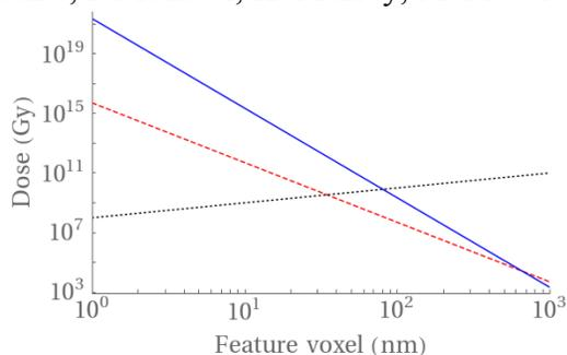
**Figure 1.** Dose required to resolve a biomolecule voxel embedded in a  $5 \text{ } \mu\text{m}$  water cell as a function of voxel size for SCXM at 64 keV (red-dashed line) and CDI (blue-continuous line) at 10 keV. The black-dotted line represents the maximum tolerable dose [2].
