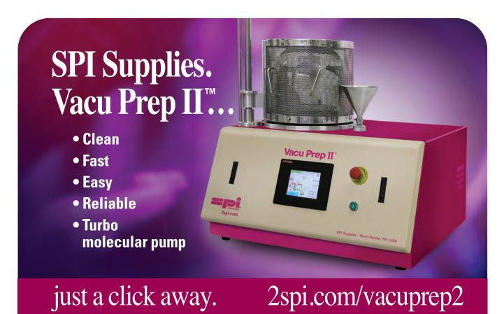
The SPI Supplies Vacu Prep II $^{\mathbb{N}}$  is a fast, clean, high vacuum, bench top evaporator with simple automated operation for evaporation or sputtering. It utilizes solid state electronics to control the pumpdown, evaporation and venting sequences. A turbo molecular pump is the heart of the system, but it still fits on the bench top.
