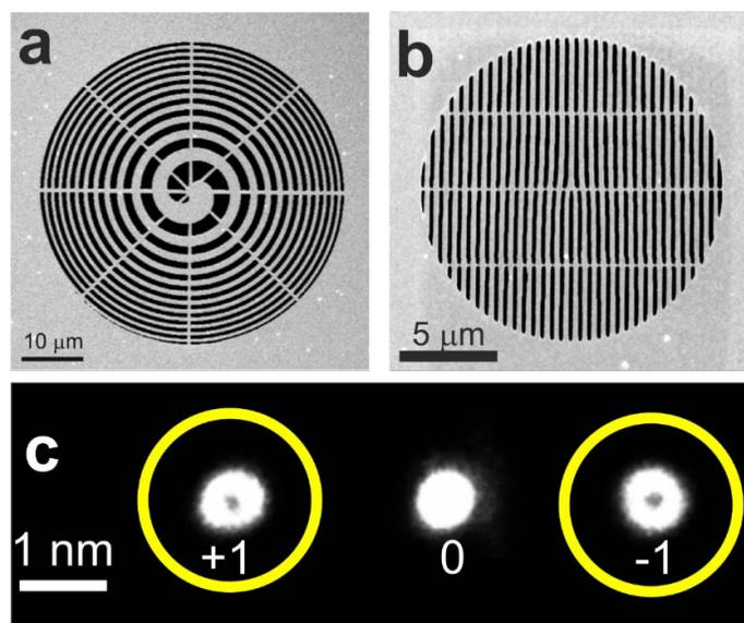
Fig 1: Generation of electron vortex beams. a, Scanning electron microscope image of a spiral-type aperture. b, Scanning electron microscope image of a fork-type aperture. c, Image of the electron beam that is generated by the fork-type aperture in b. Yellow circles mark the area of the inserted additional aperture that is used for the generation of single EVB.
