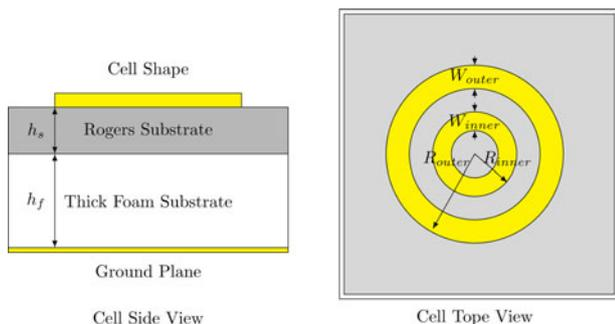
Fig. 6. Fixed beam RA antenna basic cell configuration.
