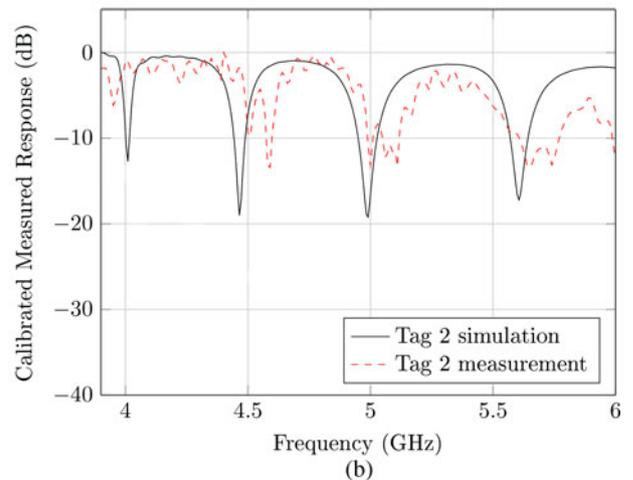
**Fig. 15.** Testbed simulation and measurement results for the first tag with code (11010101) and for the second tag (10101010).
