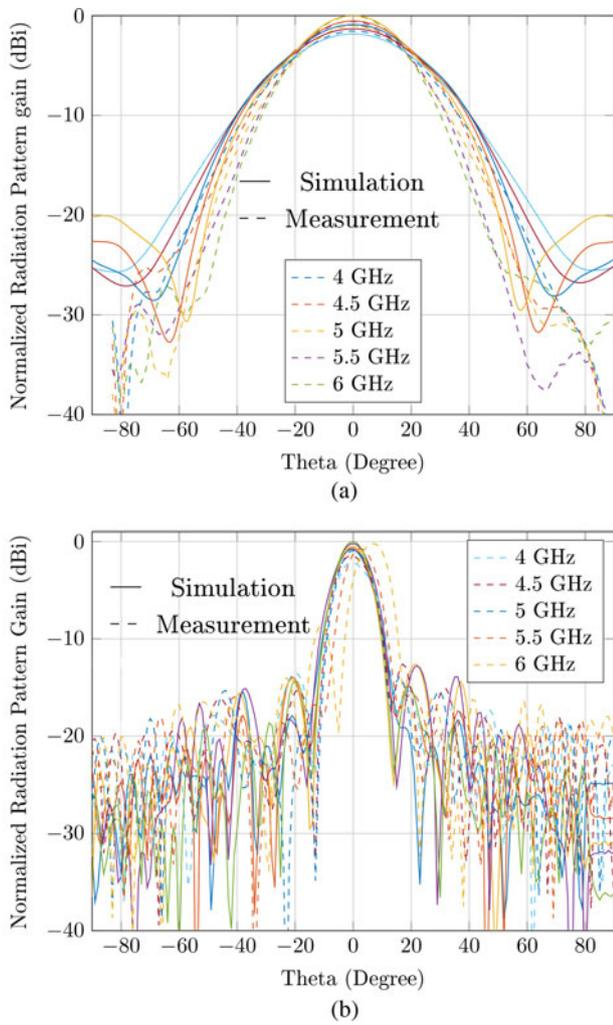
**Fig. 12.** Radiation patterns simulation and measurements: (a) Feeder simulated and measured radiation patterns. (b) Complete UWB RA antenna simulated and measured radiation patterns .
