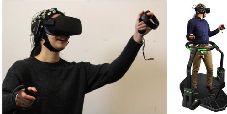
Figure 1. Off-the-shelf hardware is used in the MoBI research platform, including a VR headset, a treadmill, and an EEG cap.
