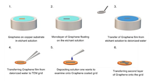
Figure 1. Procedure of making Liquid Cell
