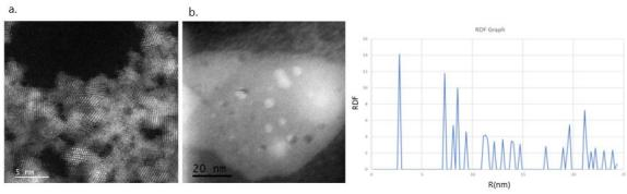
**Figure 2.** (a) High-resolution image of  $\Box\Box\Box$  fabricated by hydrolysis of ceric ammonium nitrate; (b) Image and RDF of graphene liquid cell with 1.1 mM concentration of NaCl with (-)AuNP
