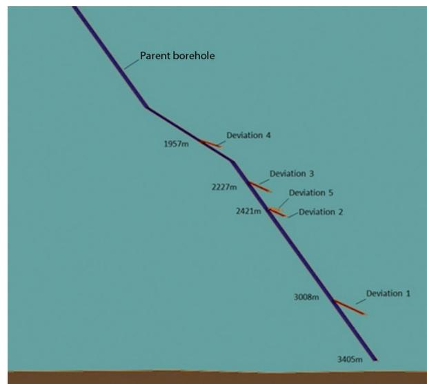
**Fig. 9.** Replicate coring borehole depiction.
