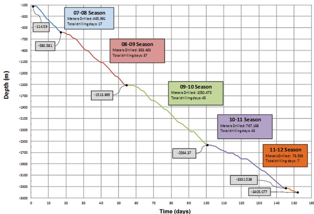
**Fig. 7.** Annual drilling progress for DISC drill borehole WDC06A, WAIS Divide Camp. Flat portions of the graph indicate Sundays off or downtime for repairs such as replacement of sheave bearings and re-termination of the drill cable.
