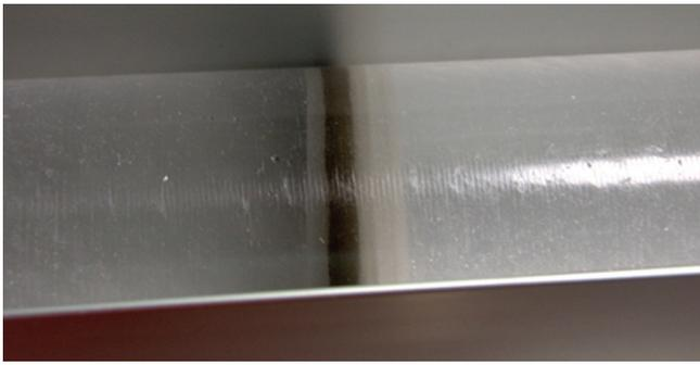
**Fig. 10.** Volcanic ash layer from 2569 m depth.
