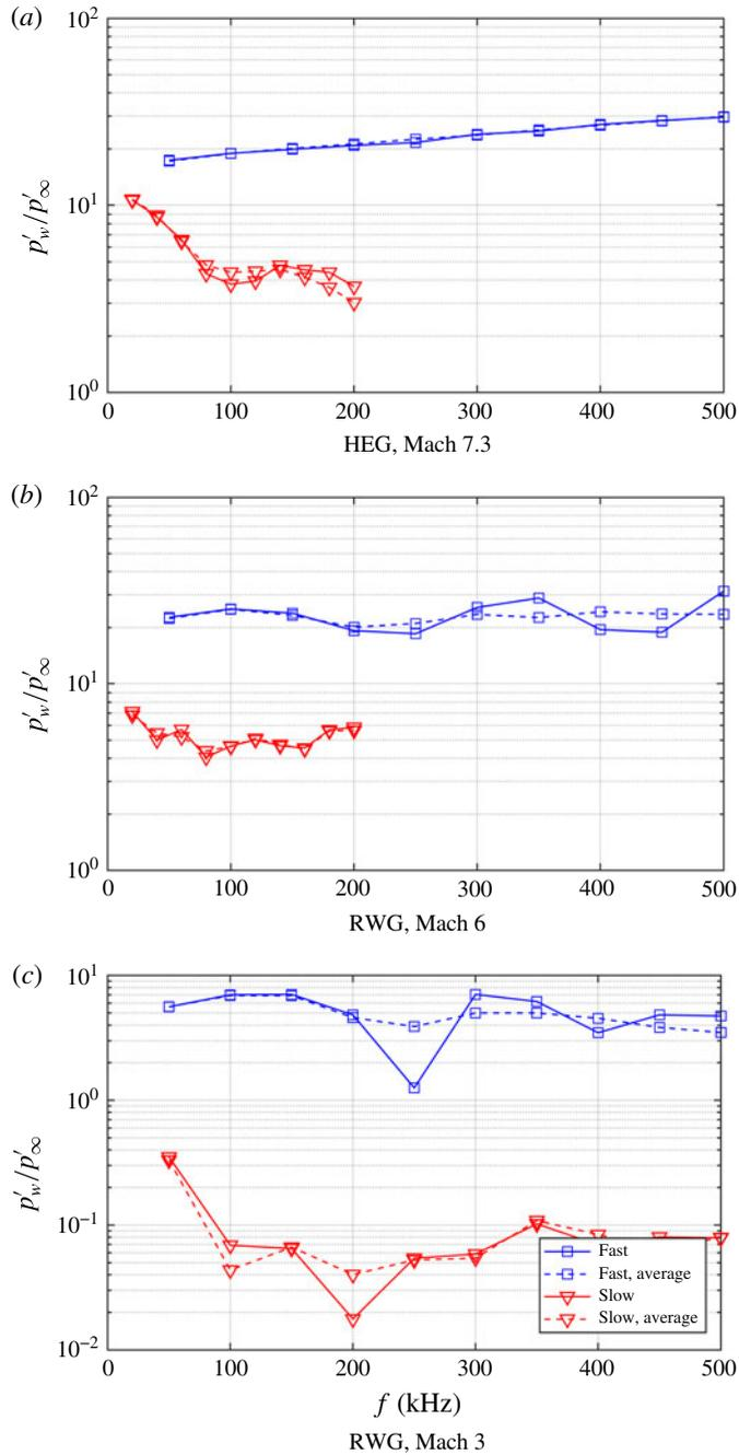
FIGURE 19. (Colour online) Frequency spectra of the pressure fluctuation amplitudes at the transducer position  $x = 29.83$  mm with both fast and slow acoustic waves, with and without spatial averaging.
