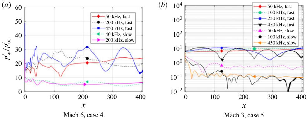
FIGURE 17. (Colour online) Pressure fluctuation amplitude distribution along the wall at the different frequencies.  $M = 6$ :  $Re_m = 6.3 \times 10^6 \text{ m}^{-1}$ ;  $M = 3$ :  $Re_m = 12.0 \times 10^6 \text{ m}^{-1}$ .
