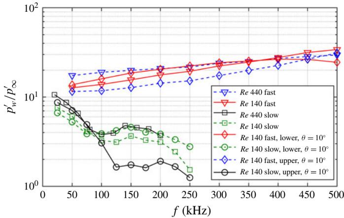
FIGURE 18. (Colour online) Frequency spectrum of the pressure fluctuation amplitudes at the transducer position ( $x = 297.3$ ) for Cases 1 to 3 (HEG) with both fast and slow acoustic waves. Mach = 7.3,  $Re_m = 4.4 \times 10^6 \text{ m}^{-1}$  (Case 1), Mach = 7.3,  $Re_m = 1.4 \times 10^6 \text{ m}^{-1}$  (Case 2 and 3). For Case 3, an inclination angle  $\theta = 10^\circ$  of the incident waves is considered.
