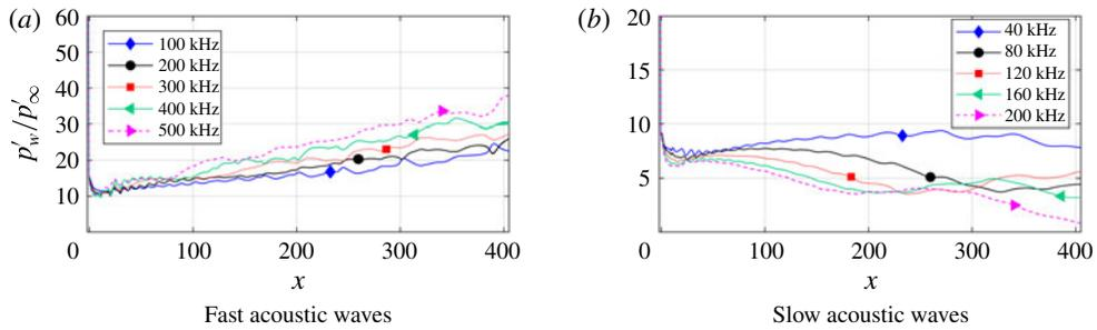
FIGURE 16. (Colour online) Pressure fluctuation amplitude distribution along the wall at different frequencies for Case 1.  $Mach = 7.3$ ,  $Re_m = 4.4 \times 10^6 \text{ m}^{-1}$ . Note that the frequency ranges were chosen differently for the slow modes.
