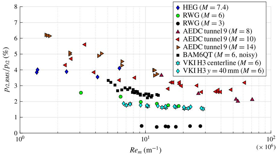
FIGURE 14. (Colour online) Normalized RMS Pitot pressure fluctuations obtained in HEG and RWG combined with the corresponding data reconstructed from Lafferty & Norris (2007), Steen (2010), Masutti *et al.* (2012) and Rufer & Berridge (2012).
