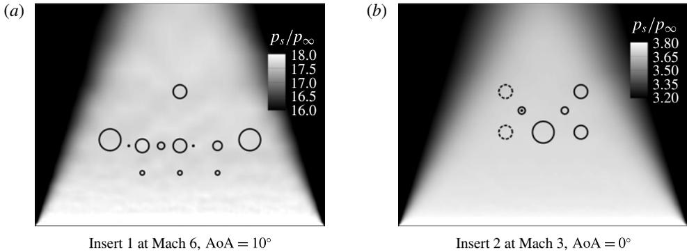
FIGURE 6. Surface pressure normalized by the free-stream static pressure on the instrumented wedge probe surface, (a) Mach 6 RWG at  $\text{AoA} = 10^\circ$  and (b) Mach 3 in RWG at  $\text{AoA} = 0^\circ$ .
