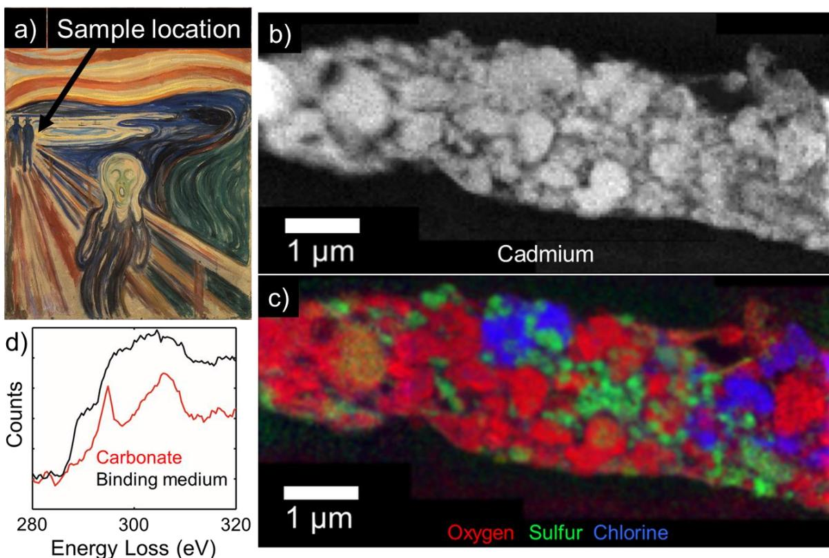
**Figure 1.** a) Approximate paint sampling location on “The Scream” indicated by arrow (Photo © Munch Museum). XEDS maps of FIBed section of paint showing b) Cadmium present throughout paint layer, and c) oxygen, sulfur and chlorine signals, which correspond to  $\text{CdCO}_3$ ,  $\text{CdS}$ , and  $\text{CdCl}_2$  respectively. d) Carbonate identity confirmed by EELS, also mapped.
