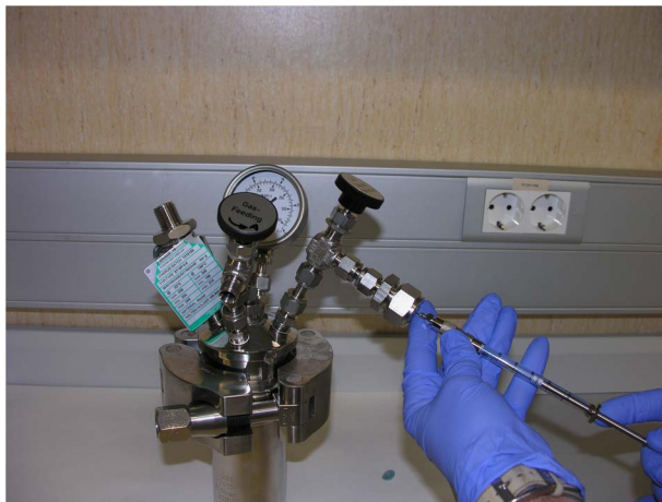
Figure 5 Gas sample extraction by a syringe.
