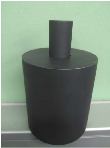
Figure 1 Pressing tool, 2 cm in diameter.
