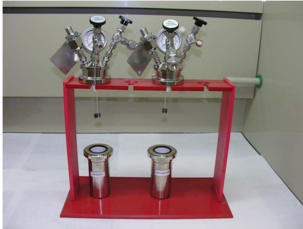
Figure 4 Leaching containers for deionized water and granitic-bentonite water.
