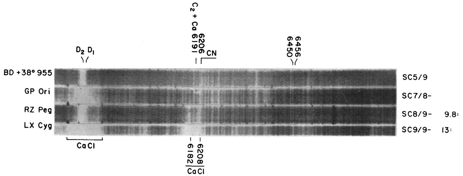
Fig. 2. Temperature sequence in the red region of SC stars. Note the ratio 6450/6456 and emergence of CaI at lower temperatures.
