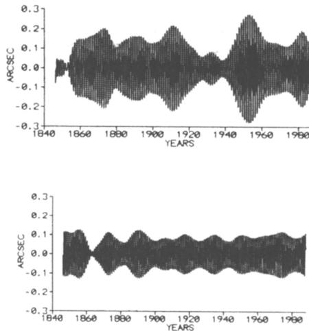
Figure 9. X components of the Chandler wobble and the seasonal variation obtained by the FT filter with widths of pass bands 1.08–1.31 and 0.93–1.09 respectively (after Nastula *et al.*, 1993).
