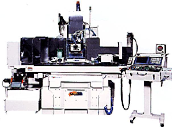
**Figure 9.** Nagase Integrex ultra high precision grinding machine.
