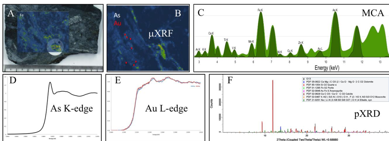
**Figure 1.** Examples of complimentary data collected at the IDEAS and CMCF beamlines (CLS). A & B mXRF maps of sample G-1-3 (overlay in A) showing distribution of Fe, As, and Au. C. Corresponding full map MCA with peak identifications. D & E As & Au XANES spectra. E. pXRD diffractogram.
