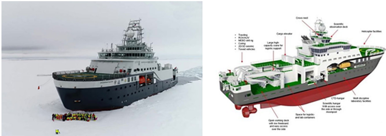
Fig. 4. (Left) The RV Kronprins Haakon in ice covered waters. (Right) Graphic illustrating specific design features and capabilities. Source: NPI.
