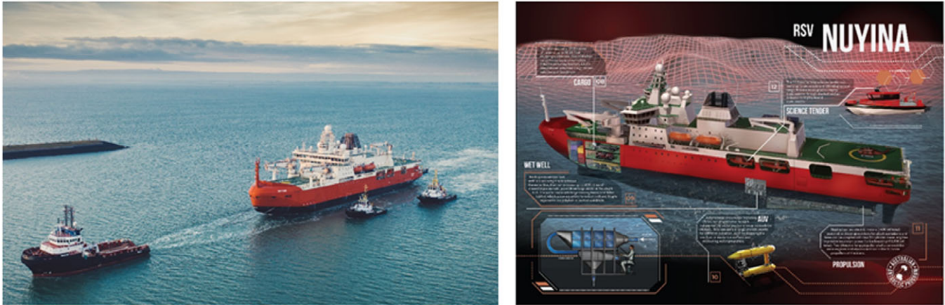
Fig. 7. (Left) RSV Nuyina under tow leaving shipyards. Source: Damen. (Right) Graphic illustrating port side design features of the vessel. Source: Australian Antarctic Division (AAD).
