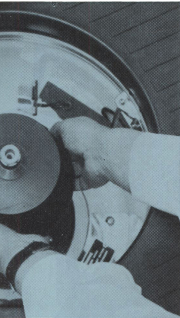
The rotor of the M.S.E. high speed centrifuge is forged by H.D.A. in a titanium alloy.
