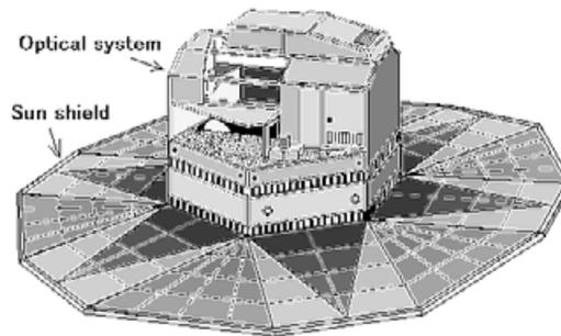
Figure 9. Schematic figure of the JASMINE spacecraft.
