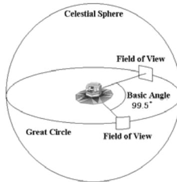
**Figure 7.** The two fields of view are perpendicular to the rotation axis and are separated by a  $99.5^\circ$  basic angle.
