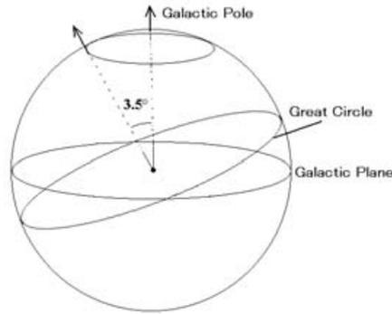
**Figure 3.** The spin axis of the JASMINE spacecraft is aligned  $3.5^\circ$  from the Galactic pole – the spacecraft line with a rotation period of about 5 hr.
