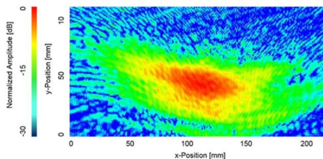
Fig. 5. Radiation pattern of the water-cooled launcher.
