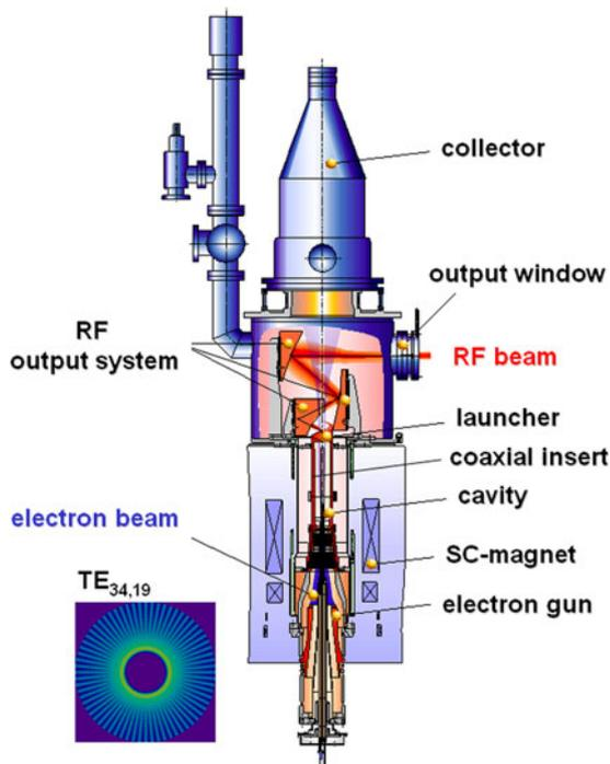
Fig. 1. Sketch of the 2 MW 170 GHz KIT coaxial-cavity gyrotron.
