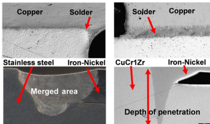
Fig. 8. Examples for grinding patterns of brazed and welded joints.
